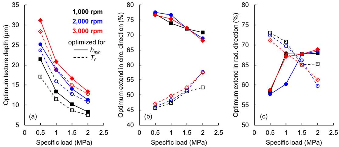
**Fig. 3** (a) Optimum texture depth, (b) optimum texture extend in circumferential direction and (c) optimum texture extend in radial direction for different operating conditions and optimization objectives.
